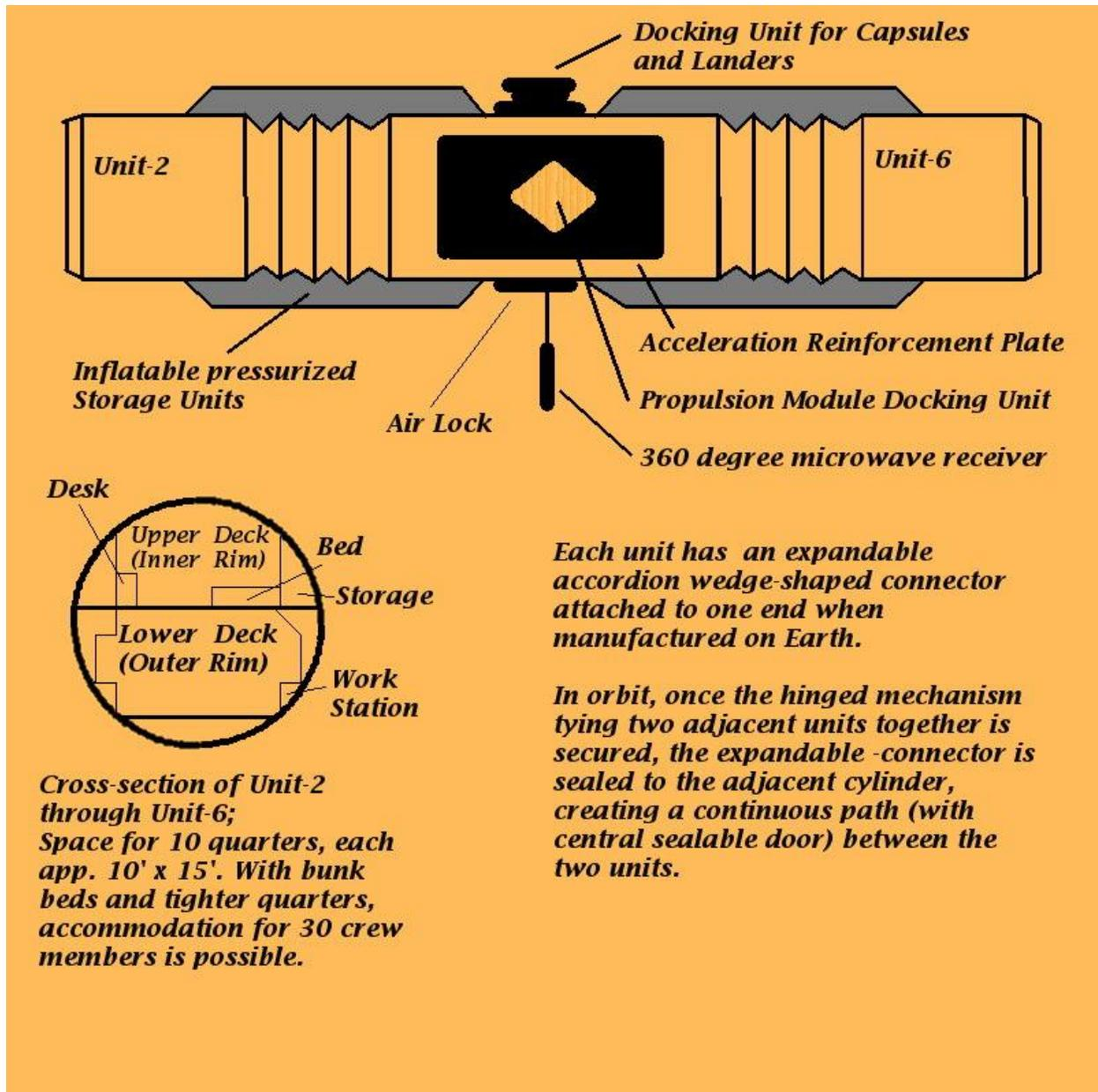
Figure 2. Side view of Crew Module and cross-section cutaway of one cylinder showing arrangement of two decks. Of course, to match the side view above, the cutaway needs to be rotated on its side.
